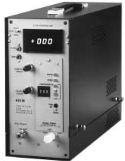
The 491MB holds the Trace Source™ Permeation Tube at a constant temperature and introduces a controlled flow of dilution gas over the tube. A small, accurate, constant flow of pure component vapor permeates from the tube and mixes with the dilution gas to form the ppm or ppb standard. The standard then flows through the generator output to the gas analyzer.
