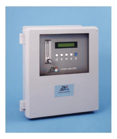
The Model IN-2000-L2-LC-W1 uses UV absorption to continuously measure ozone concentrations in the liquid phase. It uses the stripping column method with advanced electronics design, to deliver highly accurate and stable readings of dissolved ozone. The model IN-2000-L2-LC-W1 is typically used in measure dissolved ozone in drinking water, wastewater and DI water applications in a wide range of industries.
